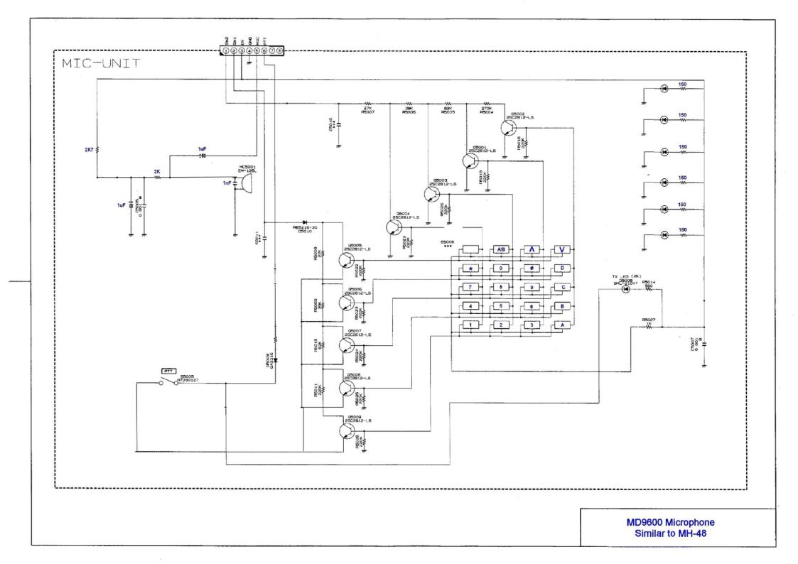
Thinking ahead to making a mobile headset microphone I decided to investigate the microphone connections for the MD9600. It appears that the microphone circuitry is almost a direct copy of the Yaesu MH-48, the service manual for which can be found on the internet.
