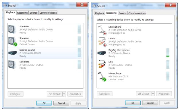
I note that there seems to be some signal coming in on the DigiRig Mic, when I unplug the audio connection on the back of the radio, that sound goes away. This is also backed up because I see the waterfall on FLDigi showing signals
